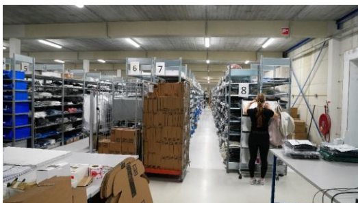
Turning the warehouse racking by 90 degrees allowed an extra 30 racks to fit into the same space: a gain of almost ten percent.
