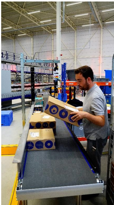
The returned goods pass through a sorter before being transported to the various workstations.
